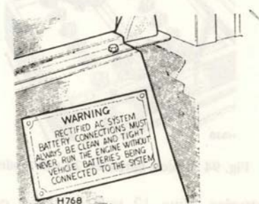
Fig. 96 Warning plate, rectified AC system, 24 volt models
