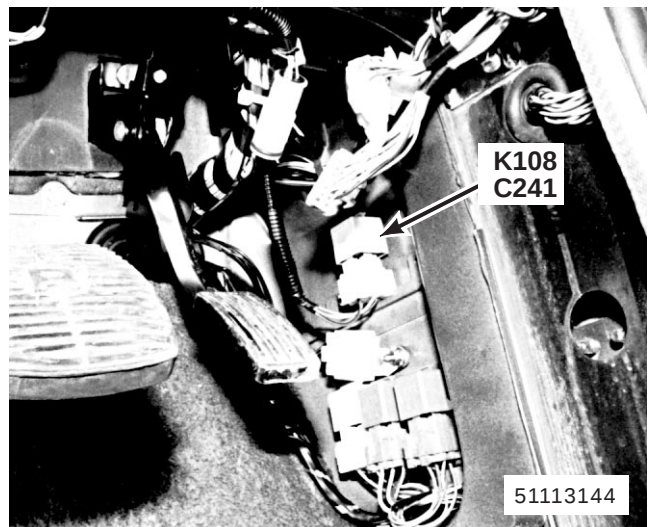
144. behind RH footwell trim panel K108 Compressor Clutch Relay C241 (5-Y)
