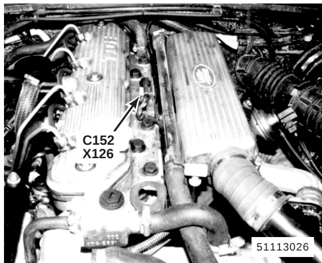
26. top centre front of engine Diesel X126 Engine Coolant Temperature Sensor C152 (2-N)
