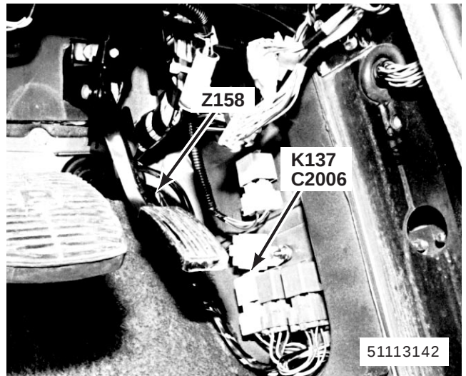
142. behind RH footwell trim panel K137 Starter Solenoid Relay Z158 Starter Relay Diode C2006 (5-Y)
